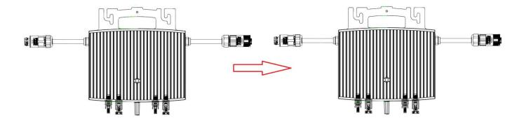
B). Install the AC end cap on the open AC connector.
