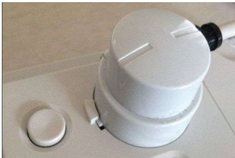
Figure 4.13.1.3 IEC1107 Optica interface with opticl communication port
