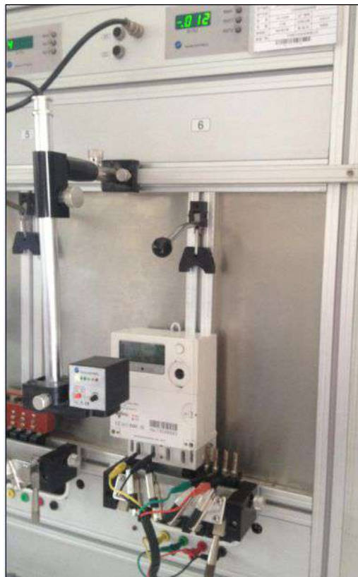
Figure 7.2.2 View of the HXE100-KP error testbench with meter
