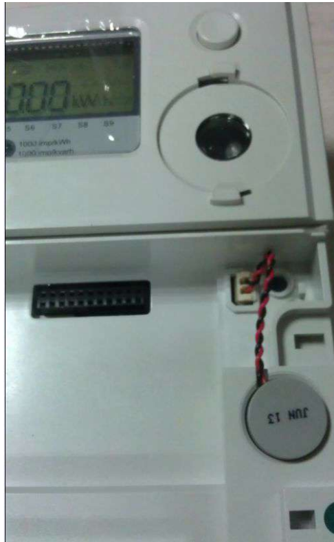
Figure 4.17.4.4 Battery installation view
