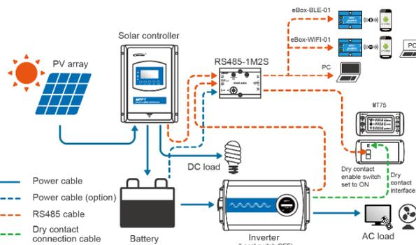
Note: When the power consumption of the external monitoring device is large, an external power connected to the auxiliary port can be used to power the device.
