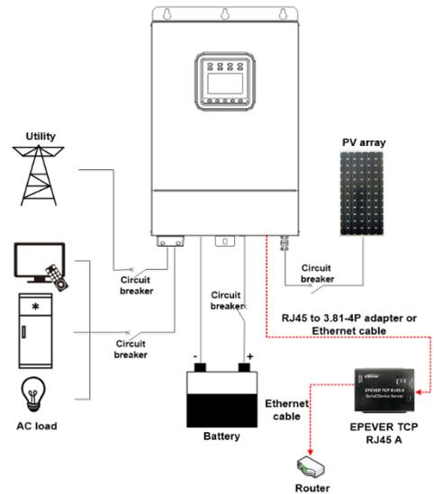
**Step2:** Login to the cloud platform (<https://iot.epsolarpv.com>) on the PC, adding the serial device server to the cloud platform. Remotely monitor the solar controllers, inverters, or inverter/charger through the cloud platforms, mobile APP, and large-screen devices. Detail operations refer to the *Cloud User Manual*.
