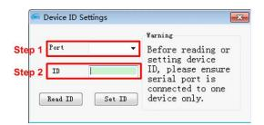
Caution: Only one of the controllers' ID can be set at each time. Follow the same procedure to set the rest of controllers.
