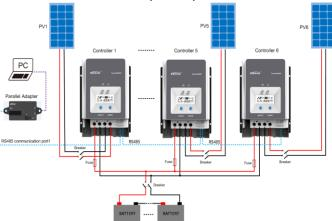
NOTE: Set each controller ID to be different before wiring (ID Range:1-10)
